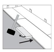
Step 4: IMPORTANT! Use hammer and tapping block to tap long edge of plank to ensure a tight fit. ANY GAPPING CAN COMPROMISE THE LOCKING SYSTEM!
