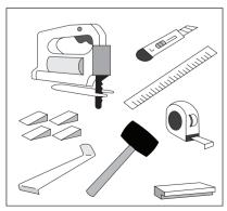
Saw, tape measure, metal ruler, metal tracing wheel, non rebound mallet and shunting tool.
