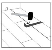
**Step 6:** Use hammer and pull bar to lock long edges of planks on final row.
