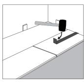
**Step 5:** Use hammer and pull bar to lock final piece in row. Insert spacer at end of row. Continue installation to final row
