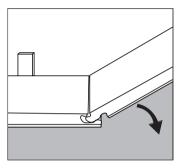
Step 2: Lock short end of plank by tapping down the ends until they lock into place. Continue to end of first row.
