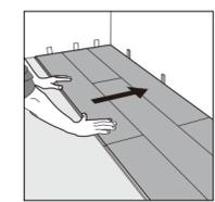
8 To lay the last row, position a loose board exactly on top of the last row laid. Place another board on top, with the tongue side touching the wall. Draw a line along the edge of this board, to mark the first board. Cut along this line to obtain of the required width. Insert this cut board against the wall. The last row should be at least 50mm (2") wide. The spacers can then be removed.
