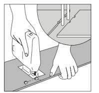
10 Holes for pipes: measure the diameter of the pipe and drill a hole that is 20mm (7/8") larger. Saw off a piece as shown in the figure and lay the board in place on the floor. Then lay the sawed-off piece in place.
