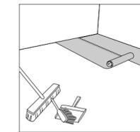
1 After thoroughly cleaning the subfloor, you should install a foam underlay (unless your product has a pre-attached pad). Run the foam underlay in the same direction as the flooring planks. The underlay should be butted side-by-side with no overlap. Tape seams together. If you are installing over a concrete subfloor, a 6mil poly (plastic sheeting) is to be installed under the foam underlay. (Many foam underlays already have this plastic sheathing pre-attached).
