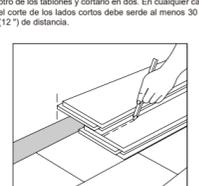
9 To lay the last row, position a loose board exactly on top of the last row laid. Place another board on top, with the tongue side touching the wall. Draw a line along the edge of this board, to mark the first board. Cut along this line to obtain of the required width. Insert this cut board against the wall. The last row should be at least 50mm (2") wide. The spacers can then be removed.
