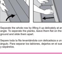
16 Disassembling / Desmontaje Separate the whole row by lifting it up delicately at an angle. To separate the planks, leave them flat on the ground and slide them apart.
