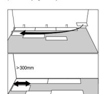
6 Lay the second row with the leftover cut part of the last plank of the previous row. This small plank should be cut to fit. Otherwise, use another plank that should be cut in two. At any case, the short sides cut are distant from at least 30cm (12").
